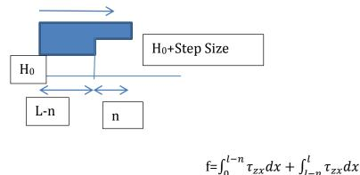
Plugging in the velocity profile from the calculations the following is obtained:
